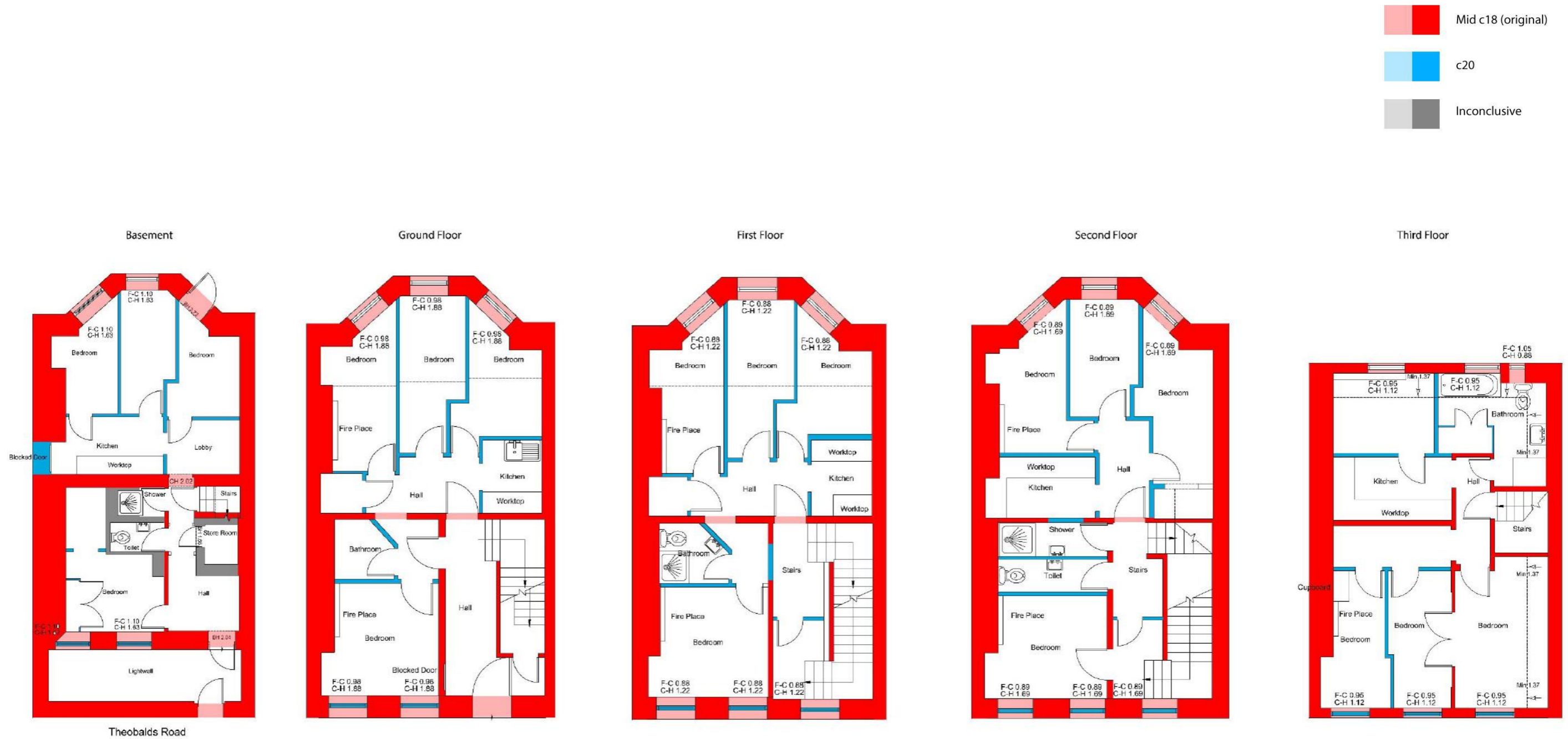
Figure 12: Morphological drawing of number 20 Theobalds Road. All external and party walls are original. The spine walls and other partitions (as indicated) are also thought to be original however there is a lack of archive evidence to confirm this. All windows on the front elevation have been replaced. It is assumed that these are mid 20 th century, possibly required as a result of war damage. The rear windows are a mixture of originals and replacements, and require further investigation. Various internal alterations have been made throughout the 20 th century, with partition walls added and altered, and additional bathroom facilities added. The origin of some internal walls is inconclusive due to the limited information available and their thickness, which is unlikely to be of recent construction.
