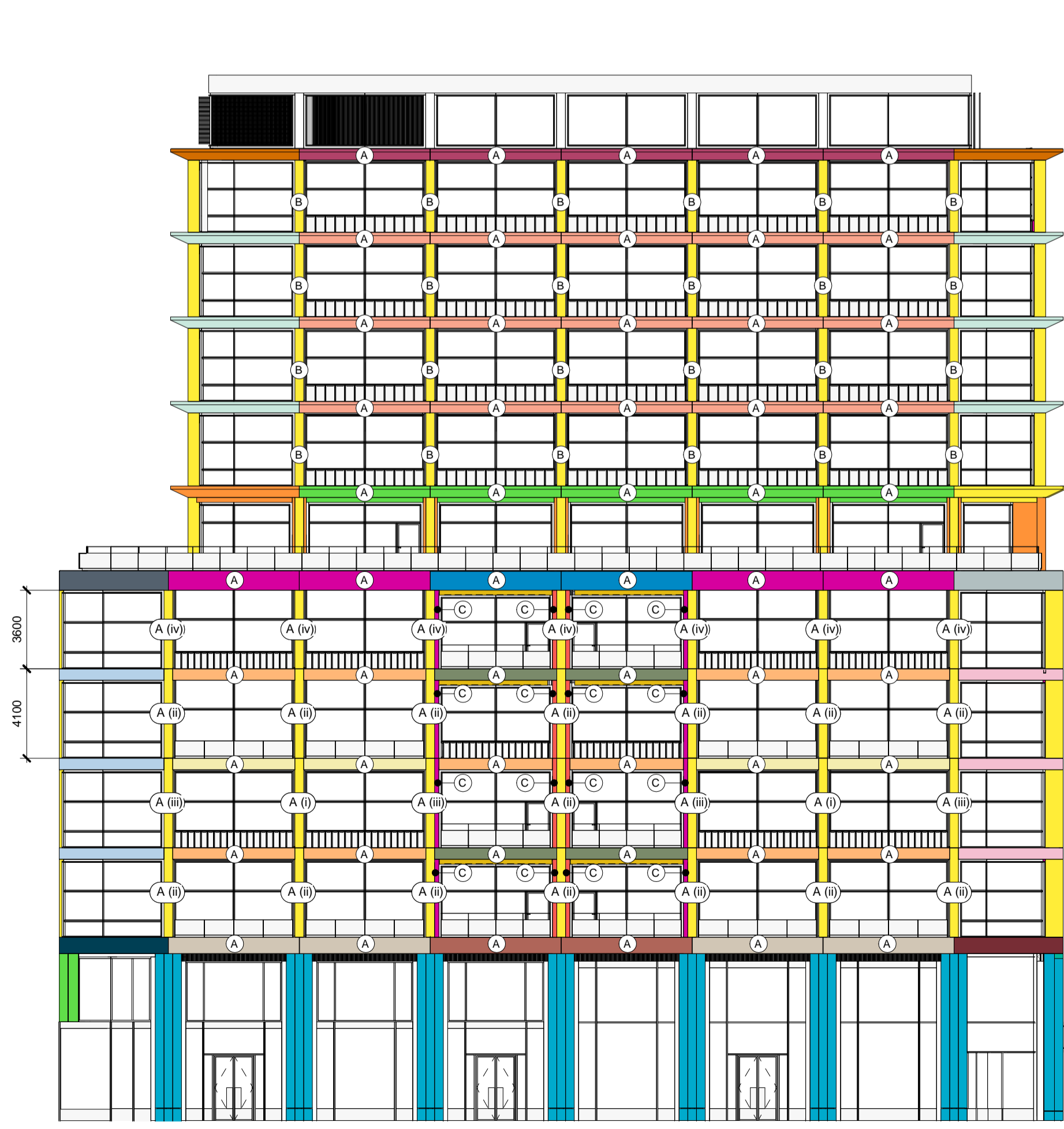
4 Concrete System - Southern Elevation 1 : 200
