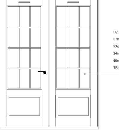
FRENCH DOORS WITH CONSERVATION PROFILE ENGINEERED SCANDINAVIAN CORE WOOD PINE RAL 9016 WHITE INSIDE & OUTSIDE 24mm BARS WITH SPACER
