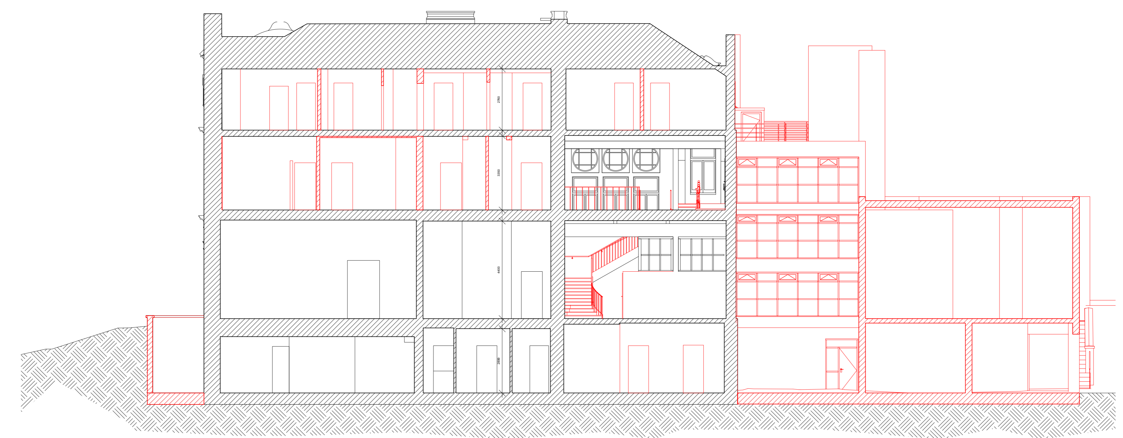
2 EXISTING AND REMOVAL SECTION E-E PL-16 Scale: 1:100
