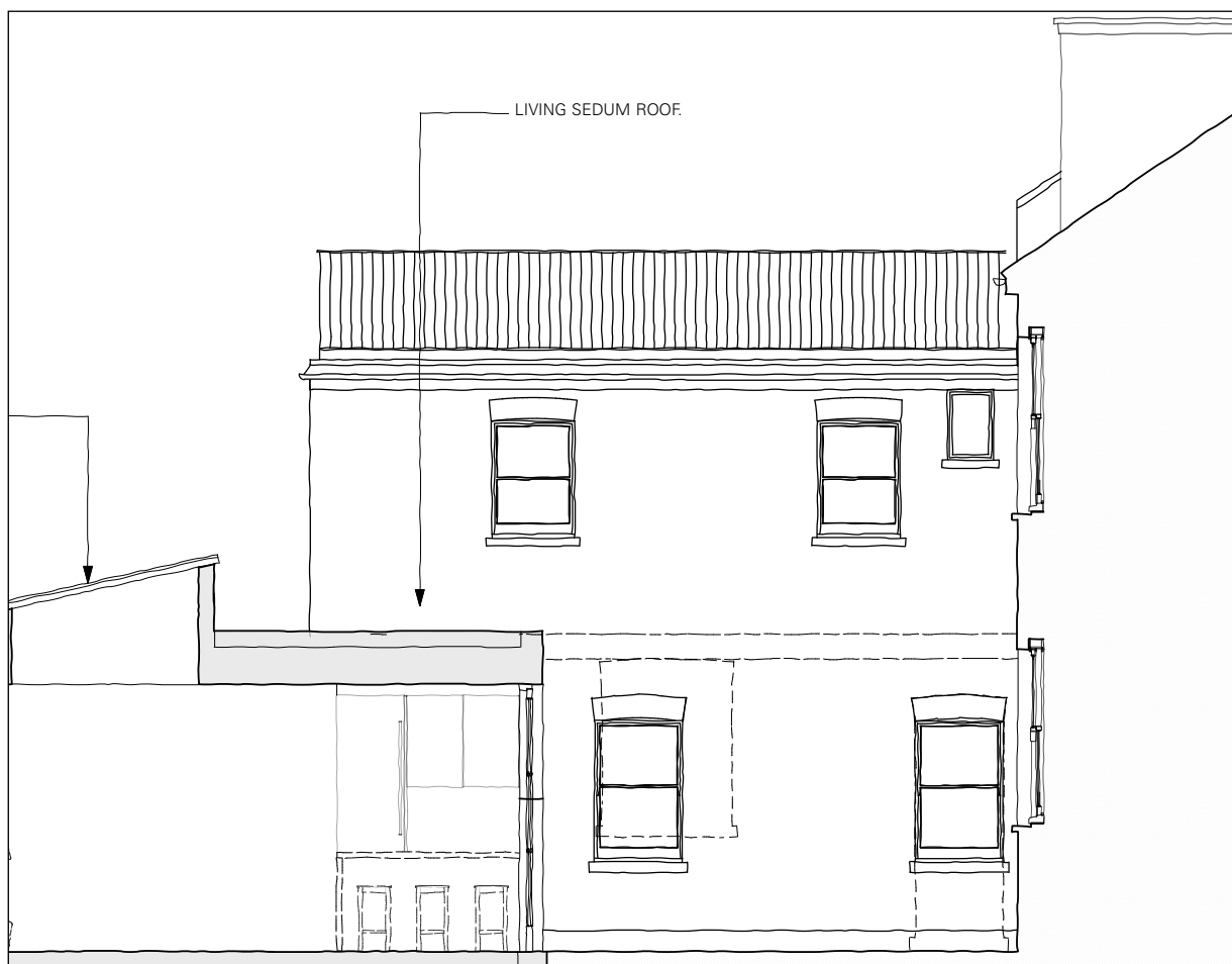
Fig 13. Part elevation/section of side return showing new windows (existing removed shown dashed) - 2019.
