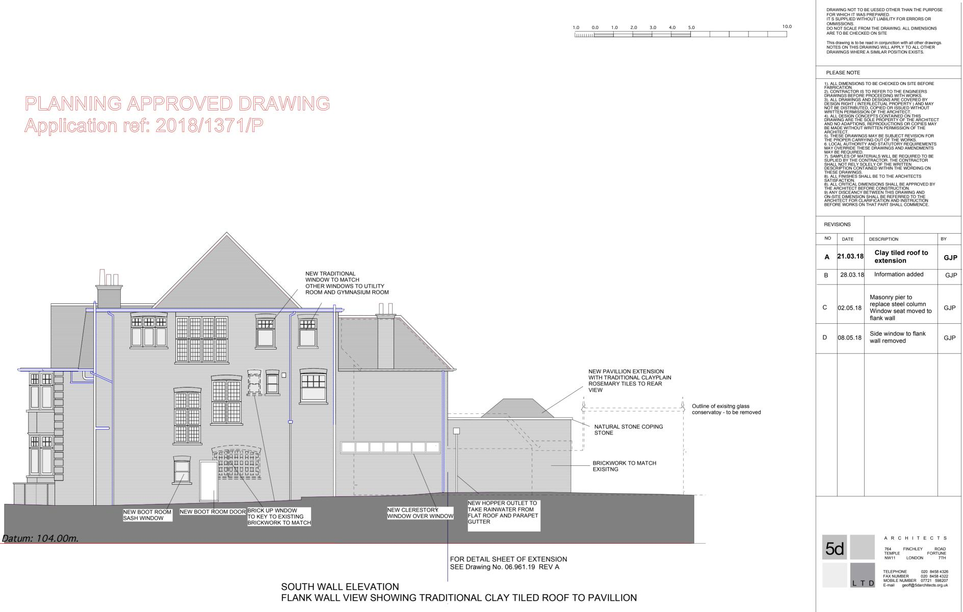
SOUTH ELEVATION - LOOKING FROM THE SOUTH PROPOSED FLANK ELEVATION
