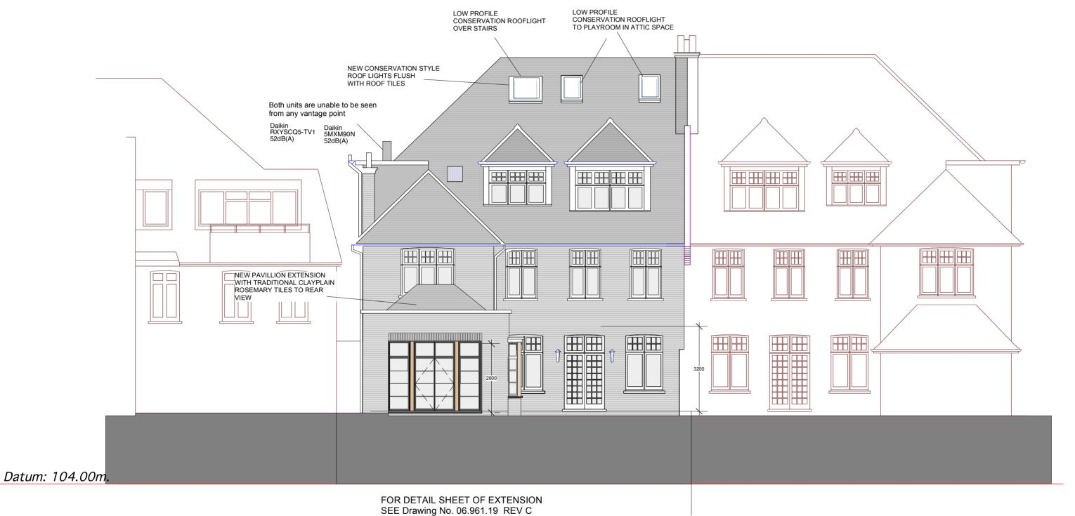
EAST ELEVATION PROPOSED REAR GARDEN VIEW SHOWING TRADITIONAL CLAY TILED ROOF TO PAVILLION DRAWING NOT TO BE UESED OTHER THAN THE PURPOSE FOR WHICH IT WAS PREPARED.
