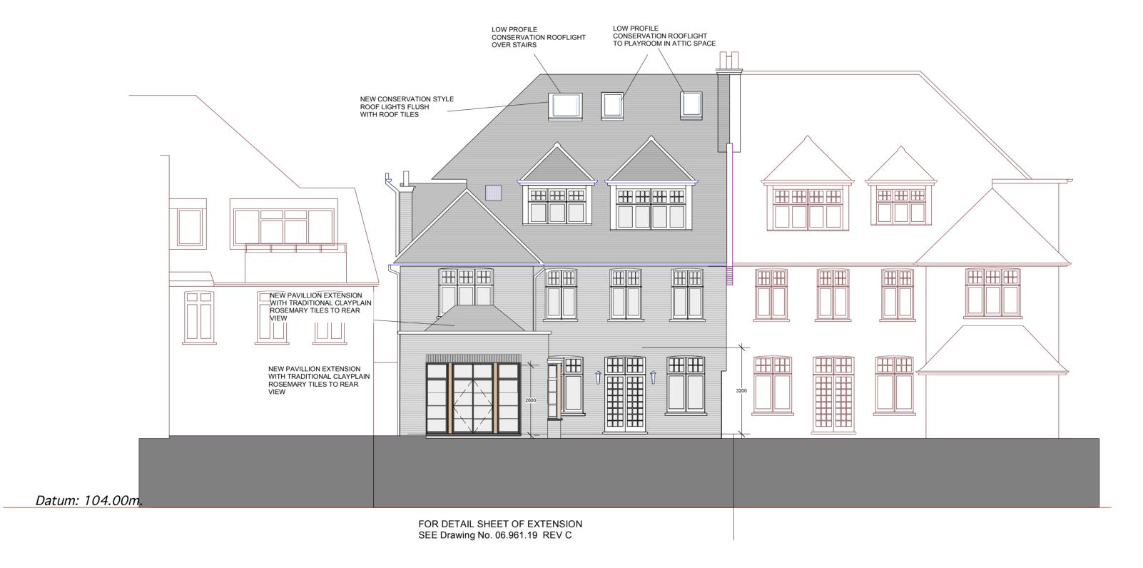
**EAST ELEVATION** PROPOSED REAR GARDEN VIEW SHOWING TRADITIONAL CLAY TILED ROOF TO PAVILLION DRAWING NOT TO BE UESED OTHER THAN THE PURPOSE FOR WHICH IT WAS PREPARED. IT S SUPPLIED WITHOUT LIABILITY FOR ERRORS OR OMMISSIONS.
