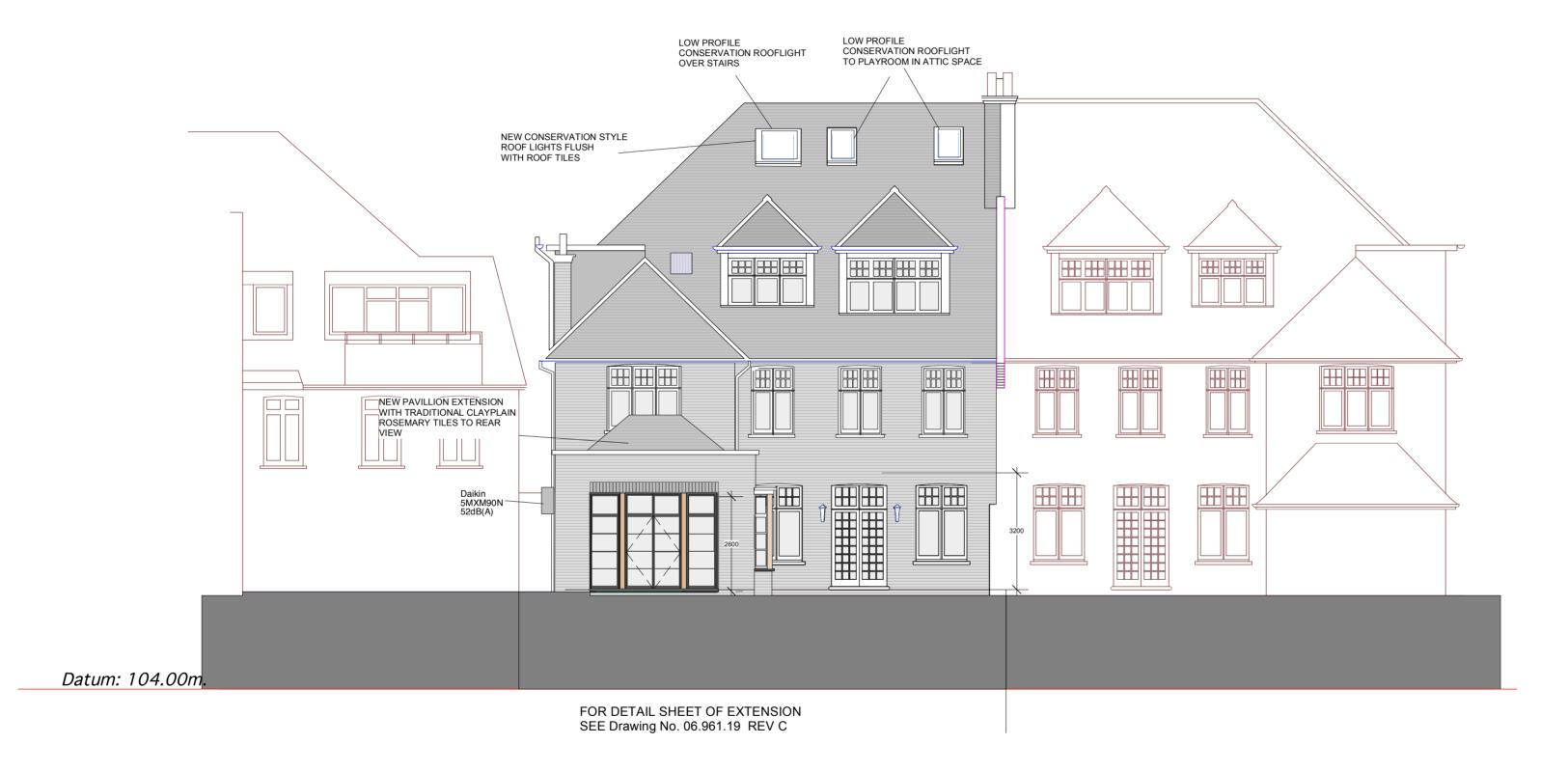
EAST ELEVATION PROPOSED REAR GARDEN VIEW SHOWING TRADITIONAL CLAY TILED ROOF TO PAVILLION DRAWING NOT TO BE UESED OTHER THAN THE PURPOSE FOR WHICH IT WAS PREPARED.
