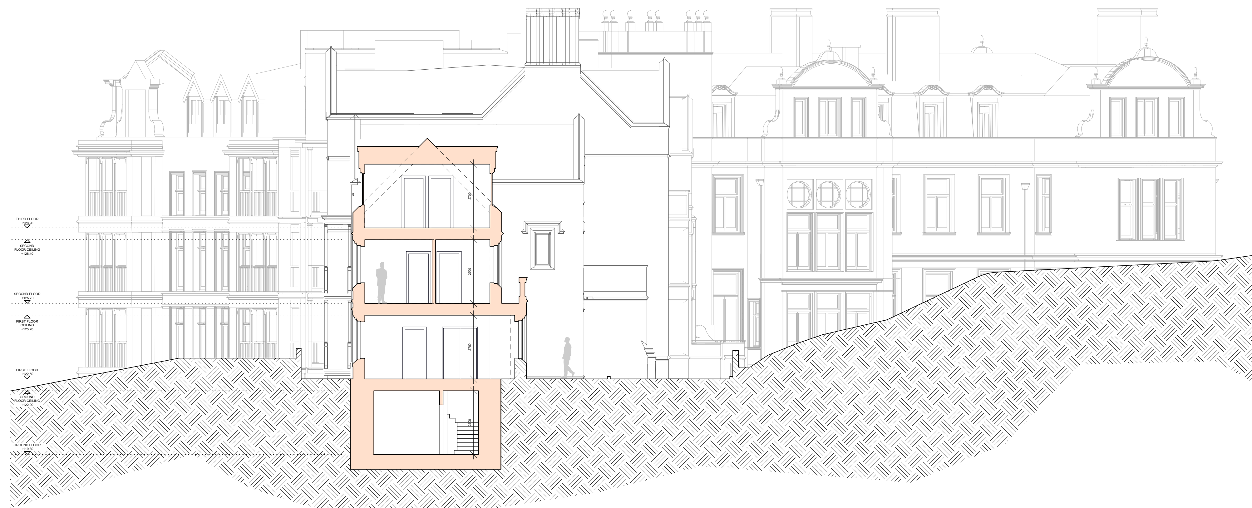
1 PROPOSED SECTION A-A Scale: 1:100
