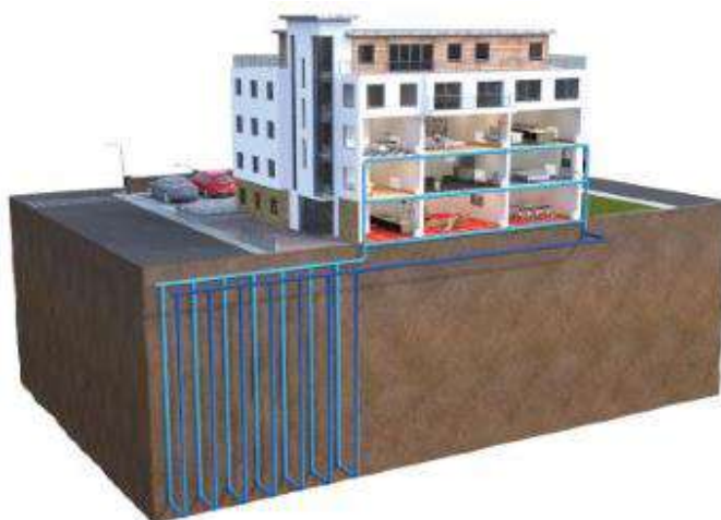
Fig 5.10 – Typical Image of Shared Ground Loop Array
