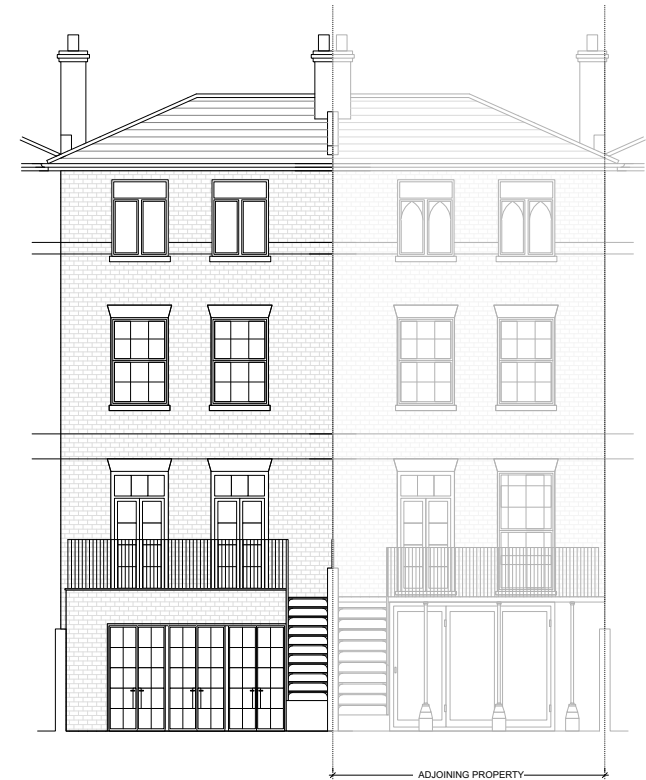
fig 15. Proposed rear elevation showing new glazing and terrace door on ground floor which are matched to the adjoining property's top floor windows and French doors respectively (not to scale)
