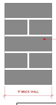
FRONT BOUNDARY WALL RECONSTRUCTED IN MATCHING FLEMISH BOND. EXISTING BRICKS TO BE SALVAGED AND RE-USED WHERE POSSIBLE. SELECTED RECLAIMED BRICKS TO BE USED TO MAKE UP SHORTFALL. NEW WALLS TO BE CONSTRUCTED USING LIME MORTAR WITH A FLUSH POINTED FINISH.
