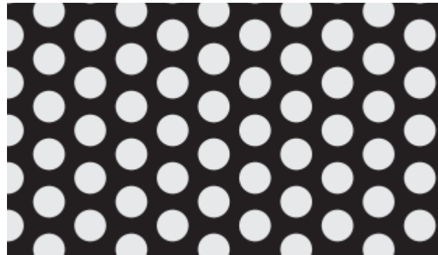
Fig. 104. Specification - 6mm DIA x 10mm pitch - 35% - To scale
