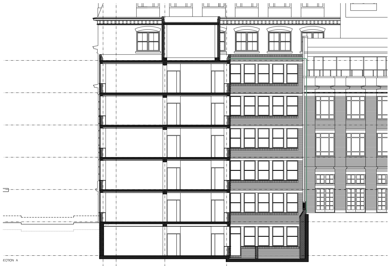
Fig. 152. Existing section with proposed infill to occupy the previous building’s site area, offering more floor space.
