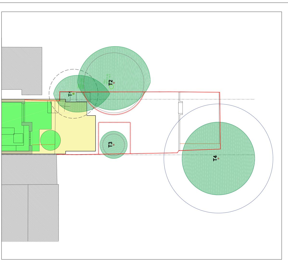
Crown spreads are represented as coloured lines that reflect the crown spread measurements indicated in the tree schedule and accord with BS 5837/2012.
