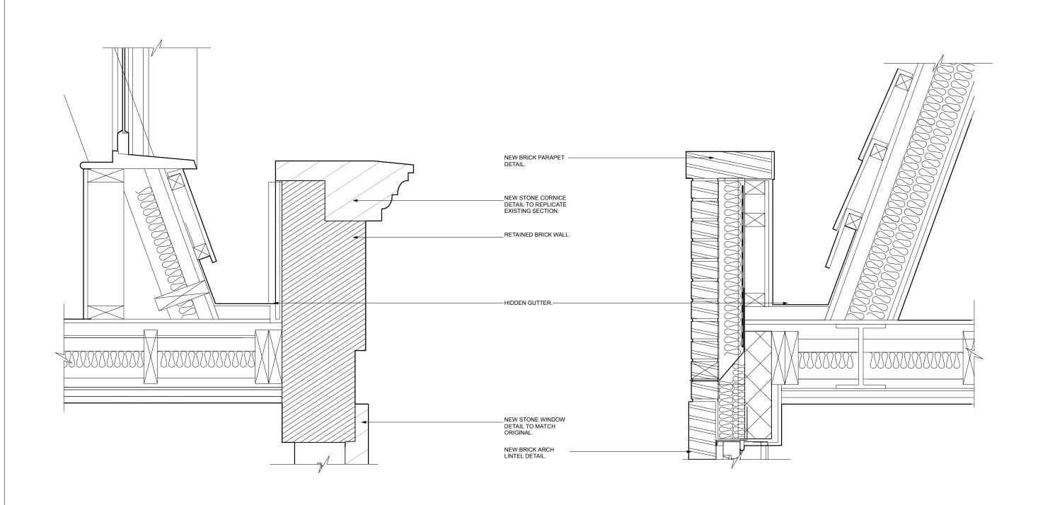
$de 52 \underset{\scriptscriptstyle{1:5@A1,\,1:10@A3}}{\text{Detail Showing Block E Parapet Cornice and Mansard Roof Junction}}$
