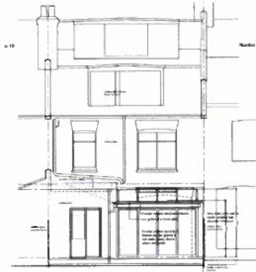
No. 17 Howitt Road Rear elevation, showing single storey rear infill extension.
