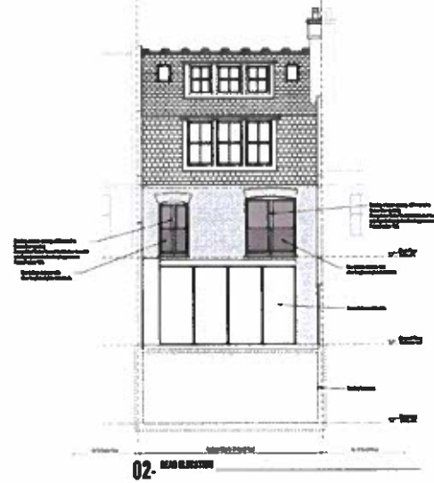
No. 21 Howitt Road rear elevation, showing 2no. Juliet balconies, approved in 2014.
