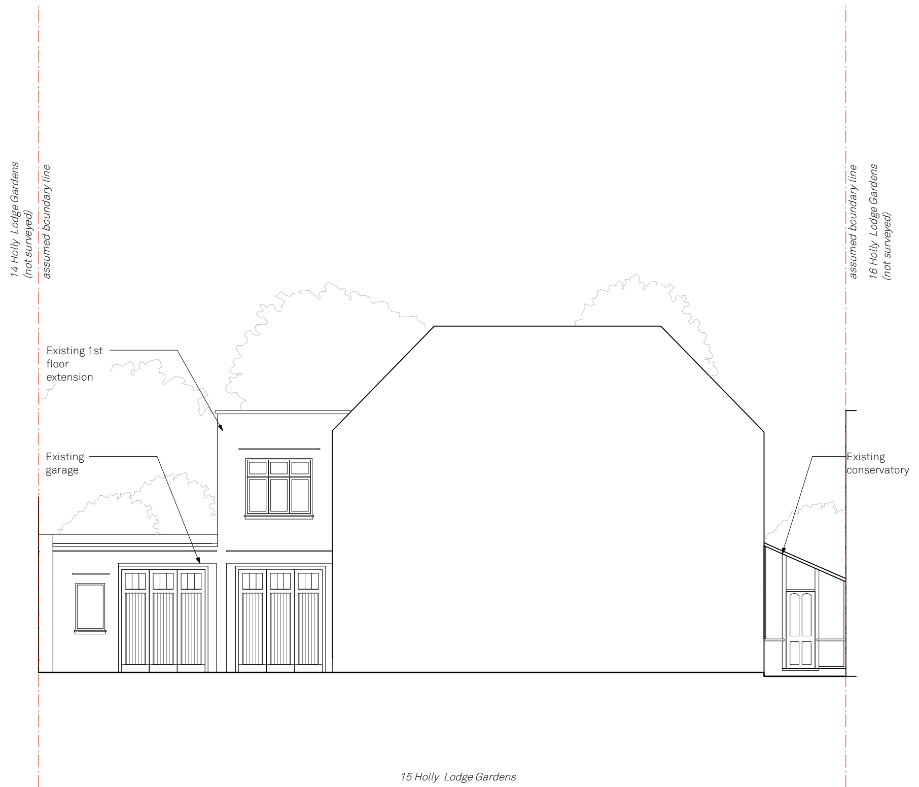
Existing Front Elevation of side extensions
