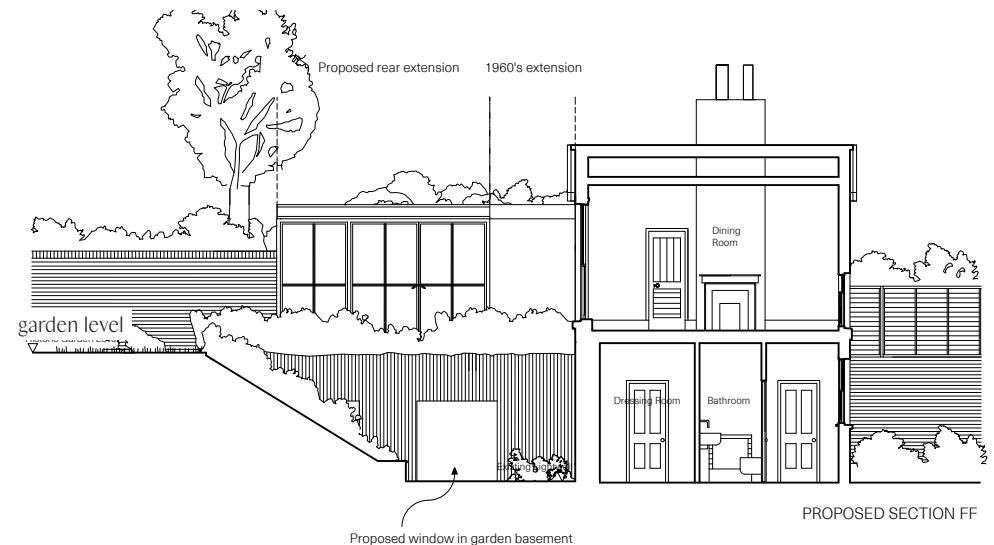
Cross Section FF through the main house and bank showing the elevation of the rear extension
