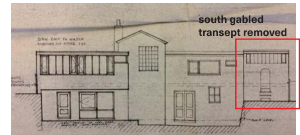
Smithsons rear elevation from RIBA archives and drawings collection dated to 1960s, shows the removal of the original 18th century transept for a flat roof
