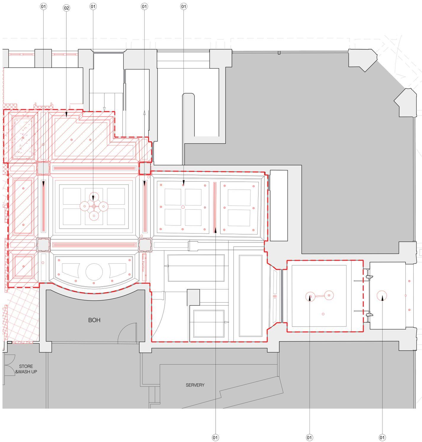
**01** Demolition Ground Floor Ceiling Plan Detail
