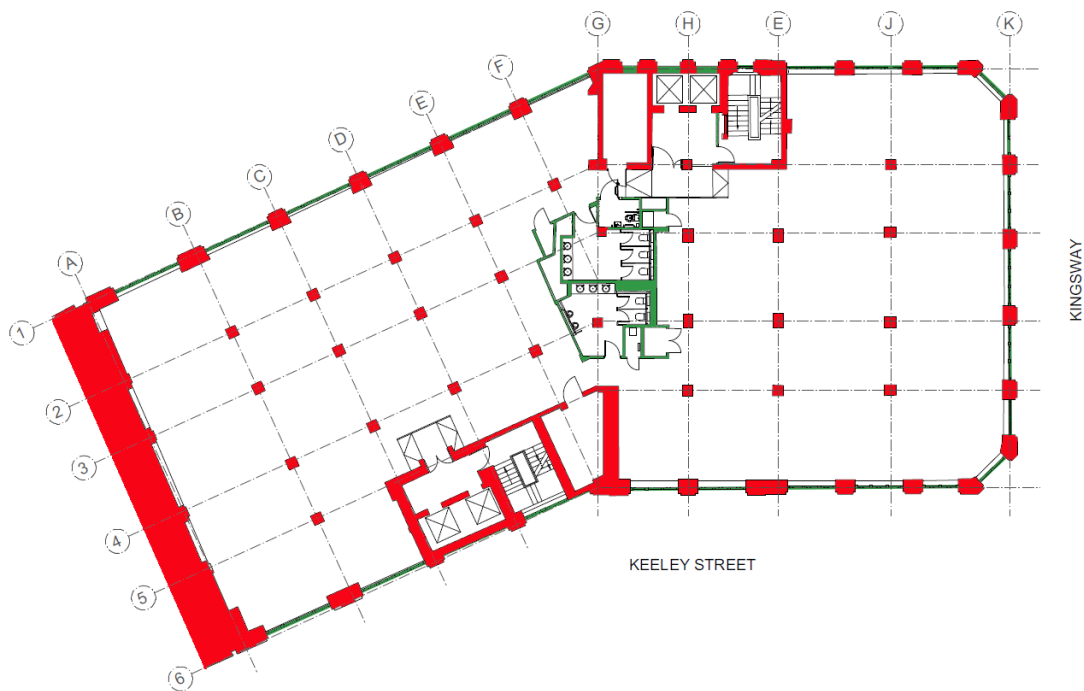
Figure 45 Second floor significance plan. Note: the second floor has been surveyed and is presented here as a typical example of the upper floor levels.
