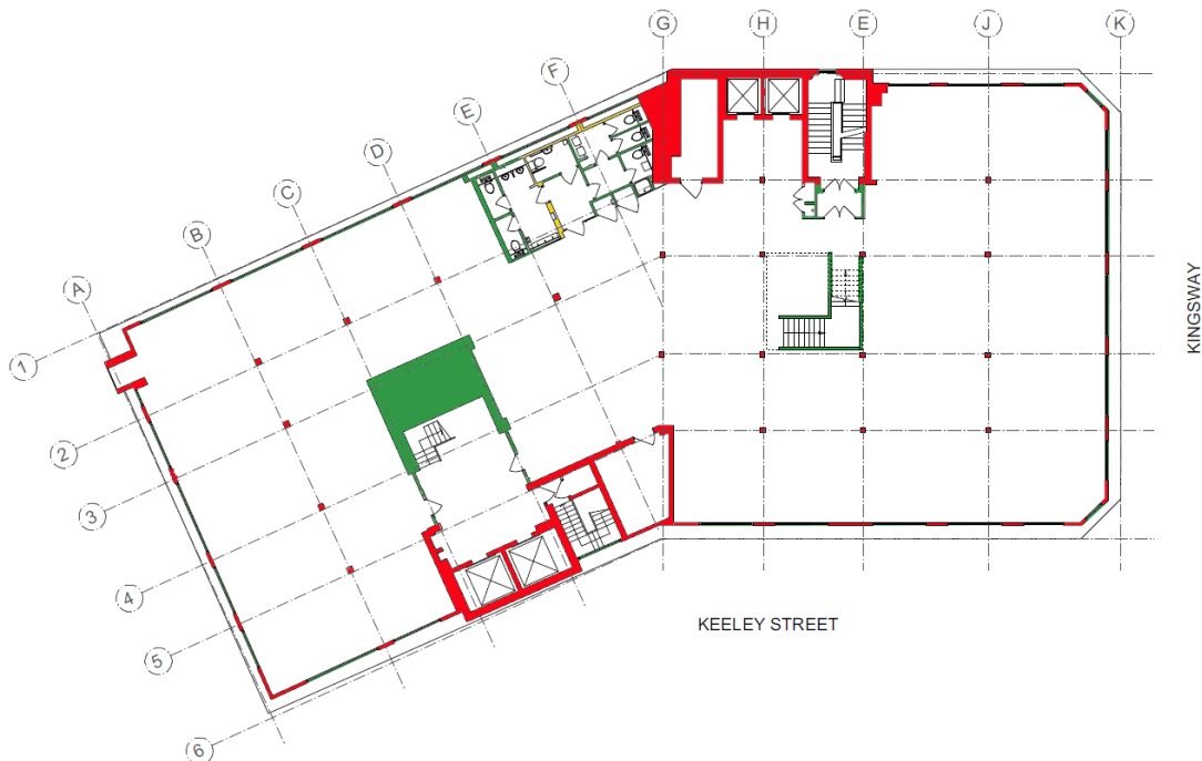
Figure 46 Sixth floor significance plan. At this level much of the alteration relates to the creation of an additional storey on top of the building including the insertion of a secondary central stair. However some of the original columns seem to have been retained.
