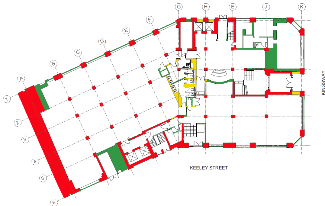
Figure 43 Ground floor significance plan. Note at this level, the entrances to the Kingsway facing shops has been moved multiple times, originally being within the marble vestibule. On Keeley Street the original loading bay door has been converted, internalising the space and an additional staircase and access point has been installed to the east of the original staff staircase. Note the enclosure surrounding the stair landings at this level have been altered, with the loss of the half the wall adjacent to the stairs.
