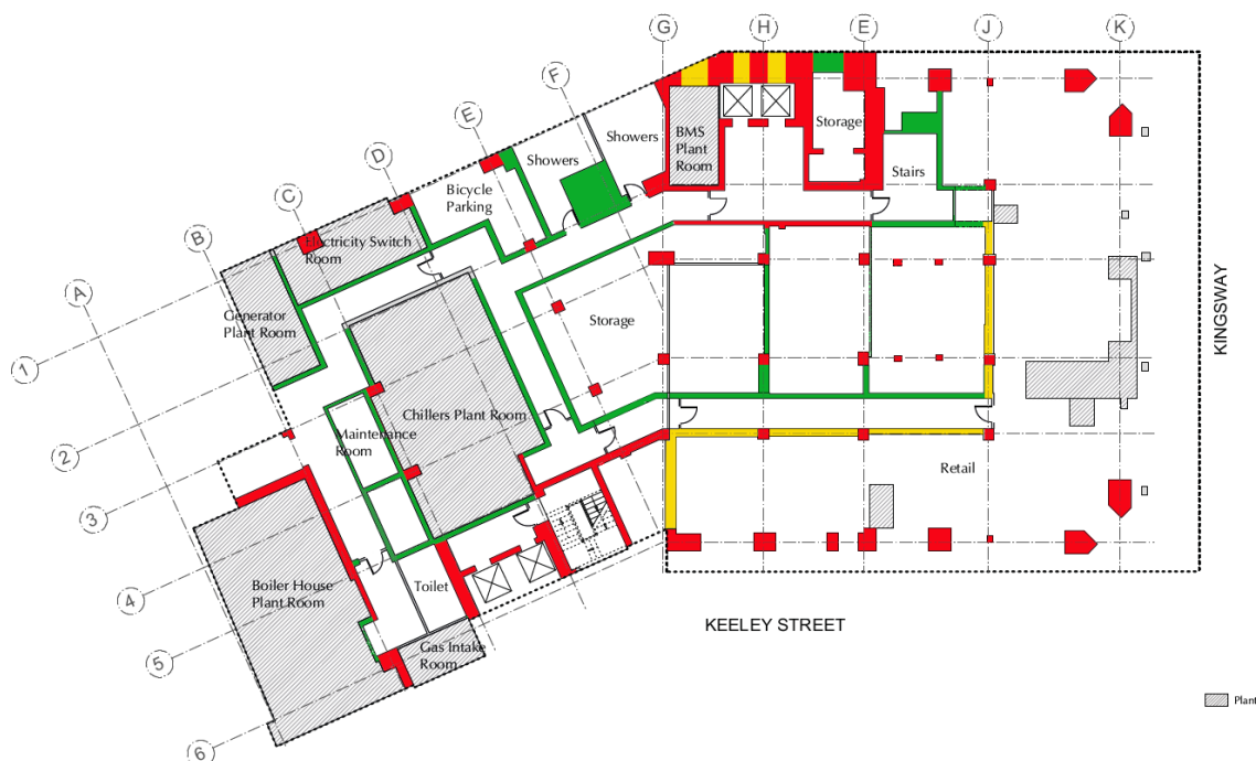
Figure 42 Basement significance plan. Note: numerous sub-divisions were installed at this level, many of which date to before 1971 and are likely to have been as a result of the building's use as an air raid shelter in 1942
