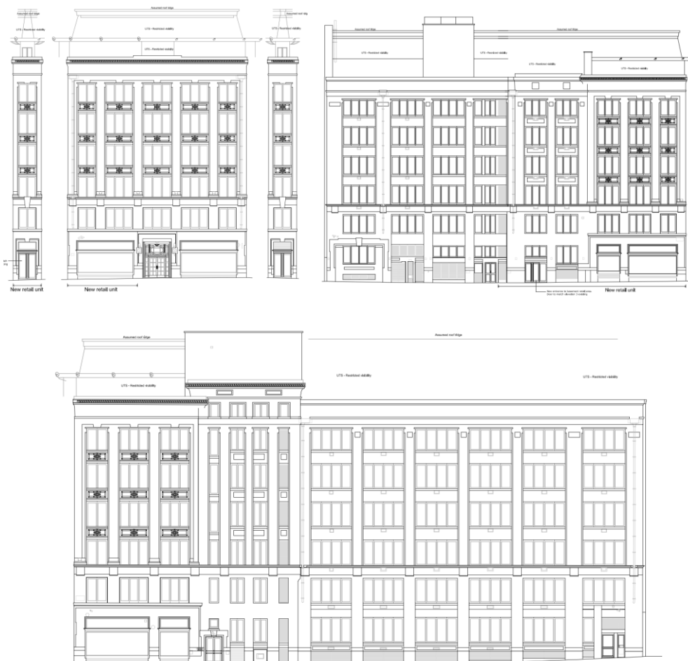
Figure 41 Extract from application 2015/4096/P showing the proposed Kingsway and Keeley Street elevations (top) and the Wild Court elevation
