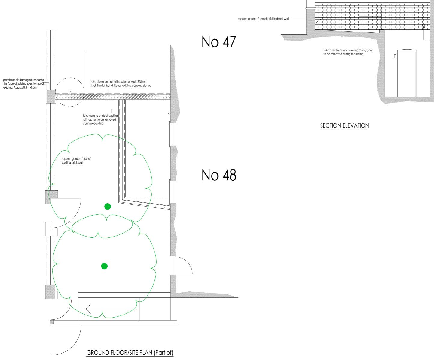
take down and rebuilt section of wall, 225mm thick flemish bond. Reuse existing coppings
