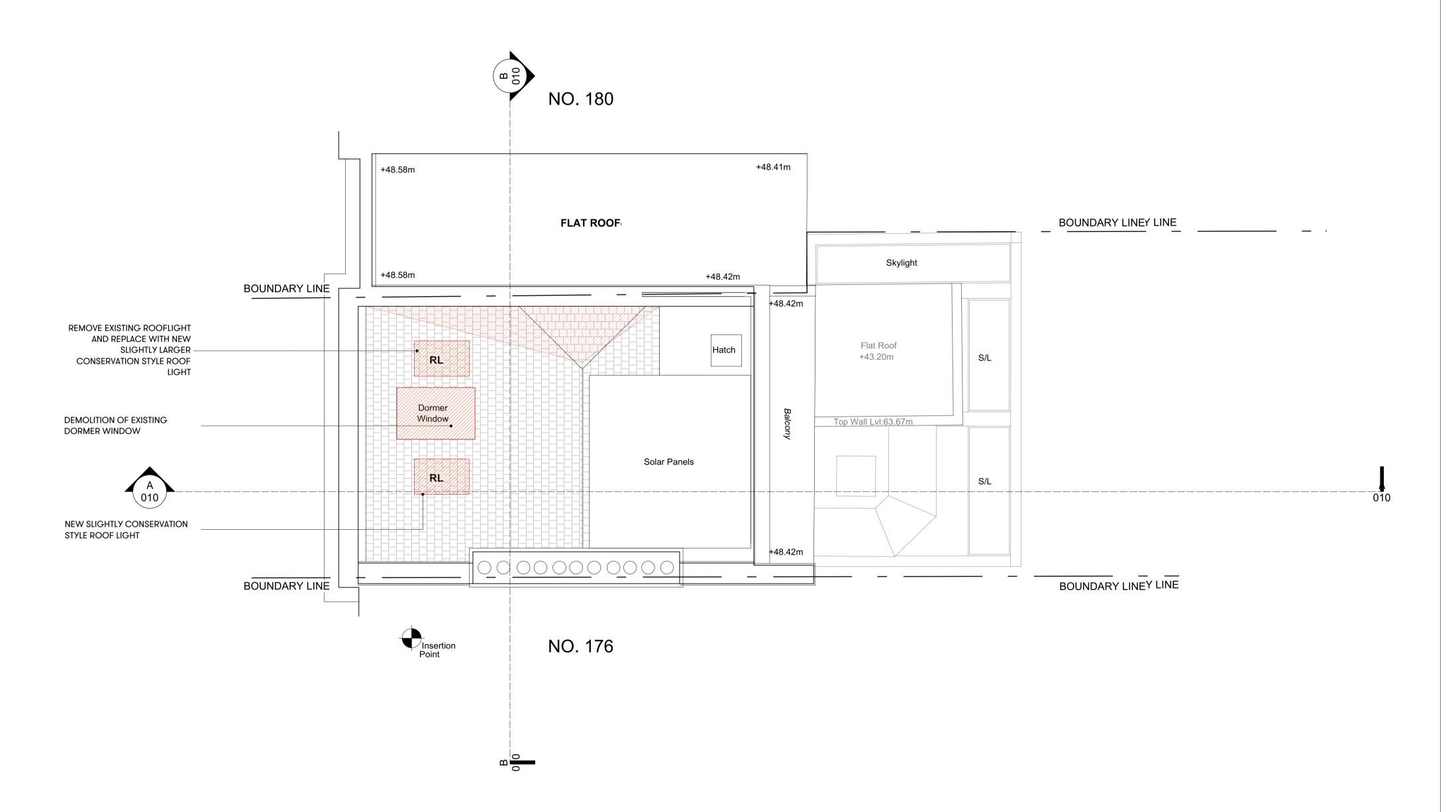
1 Proposed Roof Demolition Plan Scale: 1:50-A1 / 1:100-A3
