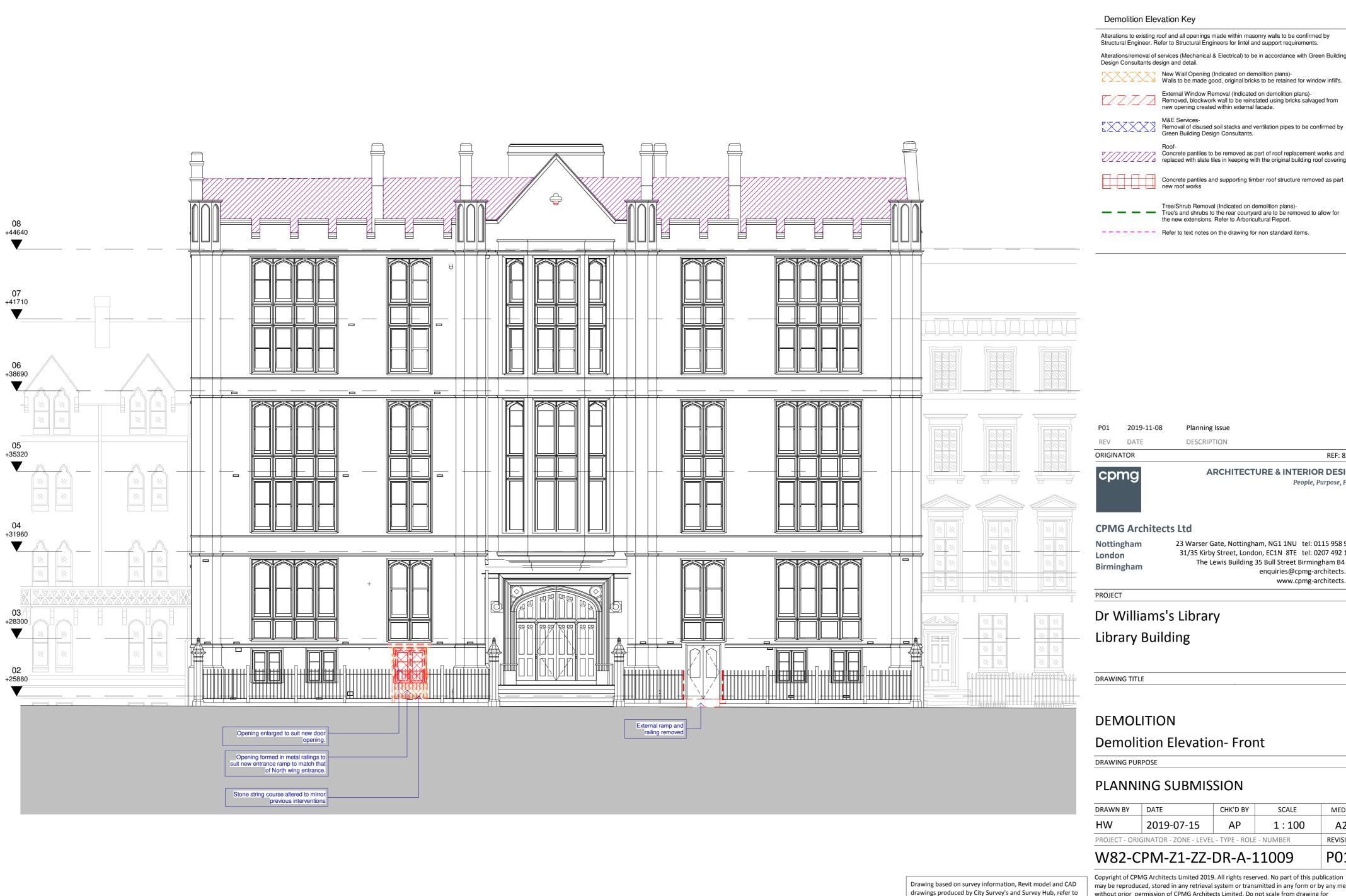
Alterations to existing roof and all openings made within masonry walls to be confirmed by Structural Engineer. Refer to Structural Engineers for lintel and support requirements.
