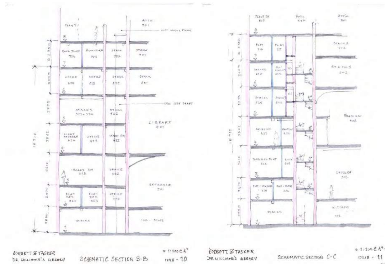
Figure 5: Sections showing existing observed structure at south wing. Left: section in east bay, looking west. Right: section in west bay, looking west.
