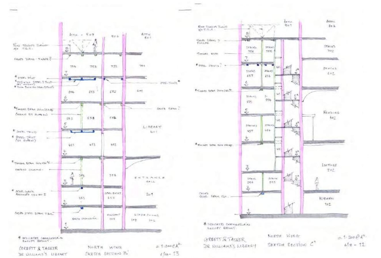
Figure 3: Sections showing existing observed structure at north wing. Left: section in east bay, looking east. Right: section in west bay, looking east.
