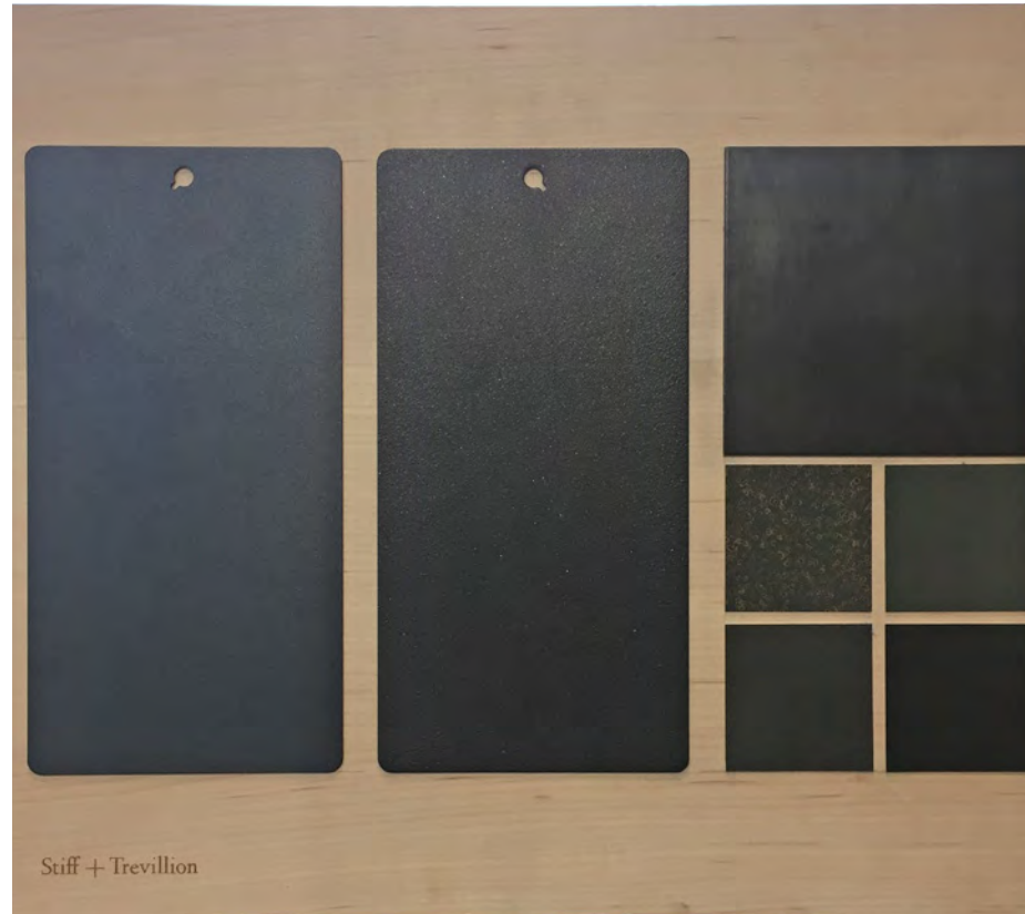
Specialist polyester powdercoat 'PPC' samples presented at DRP 'Chairs review' 8th Nov. (Potential material/colour choices Cladding type B)
