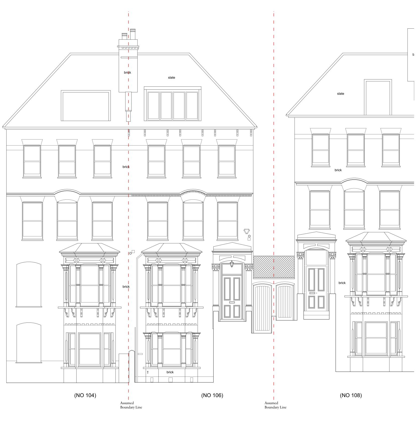
South East Elevation -Existing Building - Front Terrace Level 1 5.00 M 2.00 3.00 4.00 0
