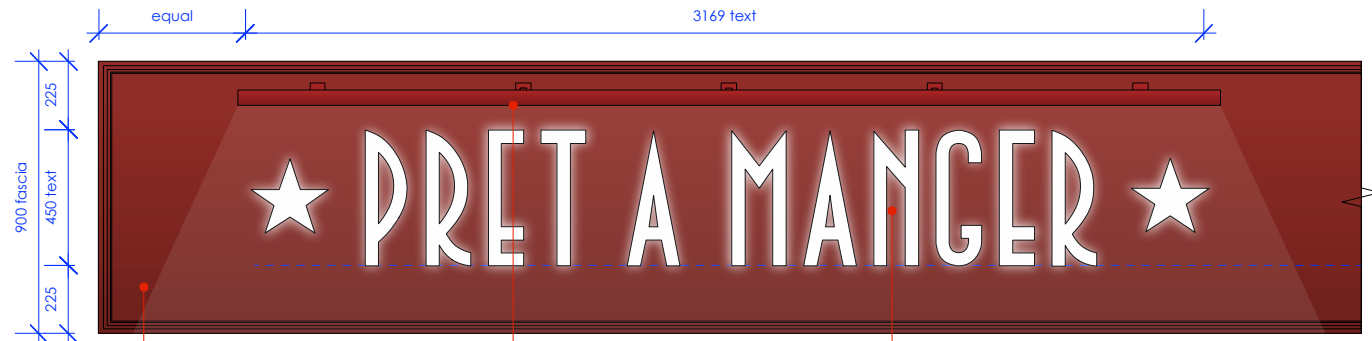
SIGN A EXTERNAL TROUGH LIT FASCIA SIGN front elevation scale 1:25
