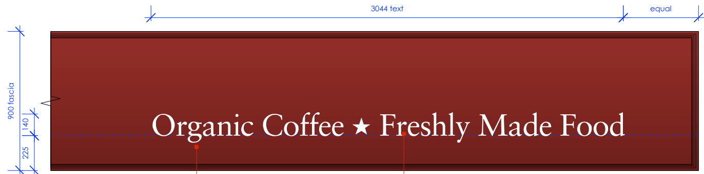
SIGN B NON ILLUMINATED FASCIA SIGN front elevation scale 1:25
