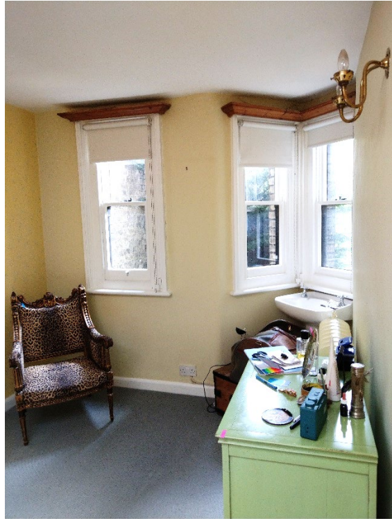
Figure 27 - Bathroom and Bedroom 2. Originally these would have been one room off the circulation corridor between the main staircase and the North Wing, these rooms were formed in the 1950 subdivision and the Minton tiles have been removed within these spaces. Original doors have been reused in modern frames, but no other internal finishes have been retained. The window was modified in the bathroom to create a smaller unit with space for an extract above. Proposals are for this to be reinstated, to match the other windows in the group.
