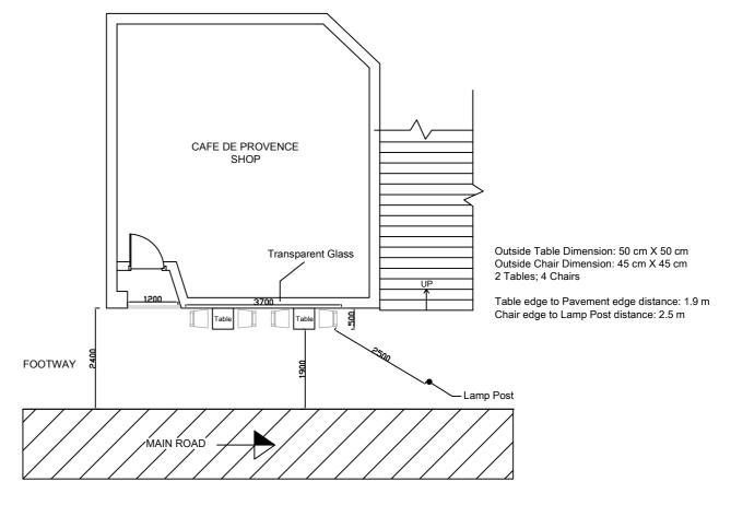
PROPOSED FLOOR PLAN WITH PAVEMENT
