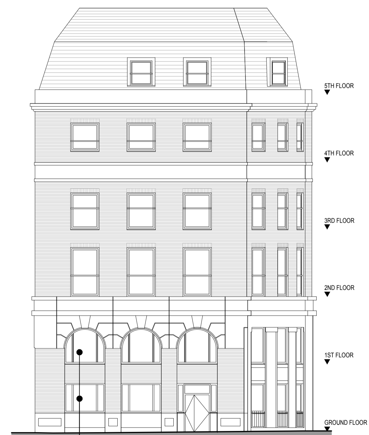
03 ELEVATION C: TO PORTPOOL LANE SCALE: 1:125 (A1)
