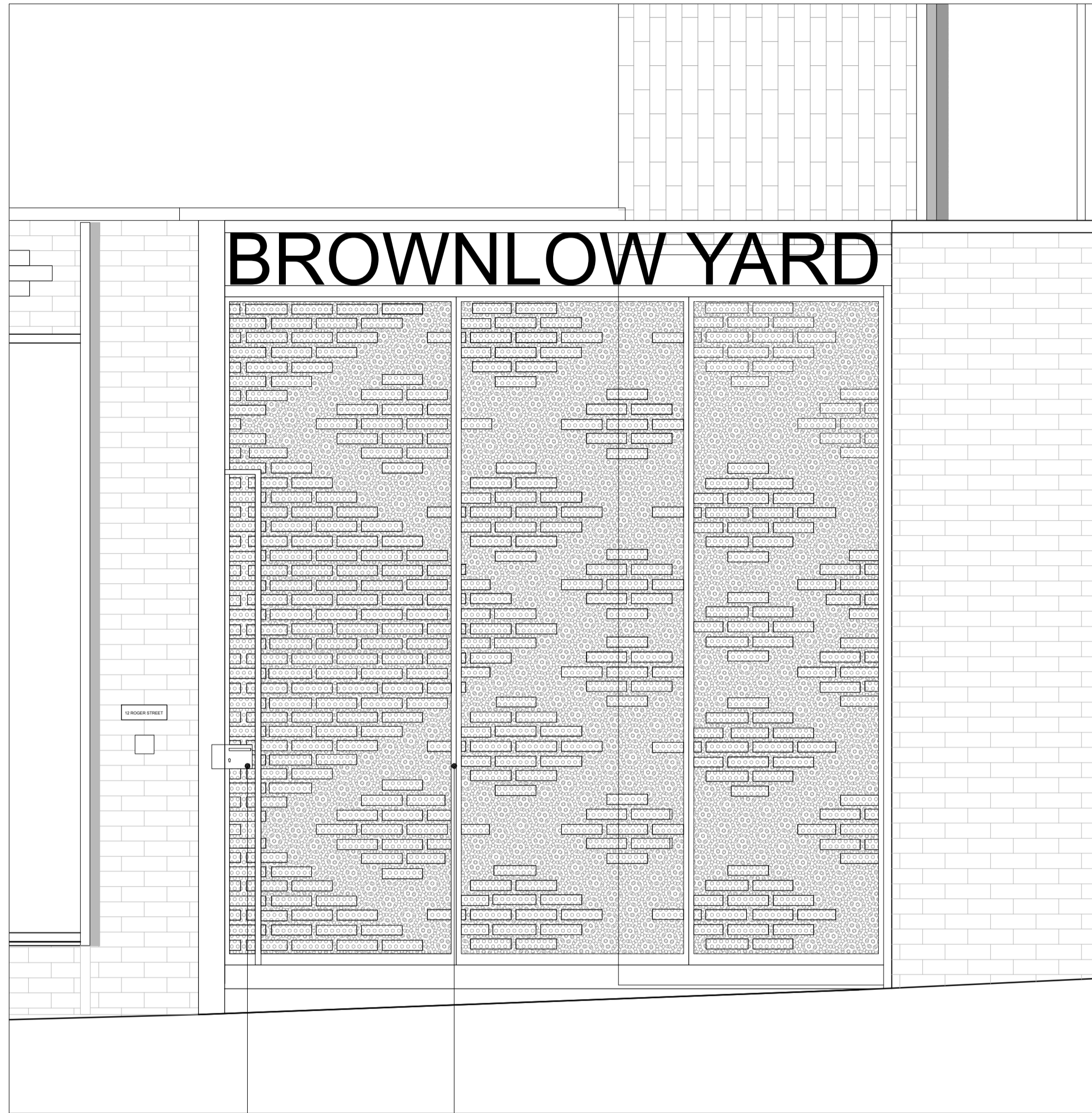
2 PROPOSED GATE ELEVATION 1:20 @ A1
