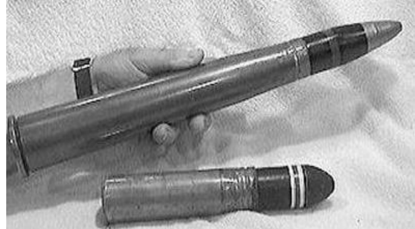
Typical shell and rocket fuzes (Above left Proximity Fuzes found by MACC in 2017)
