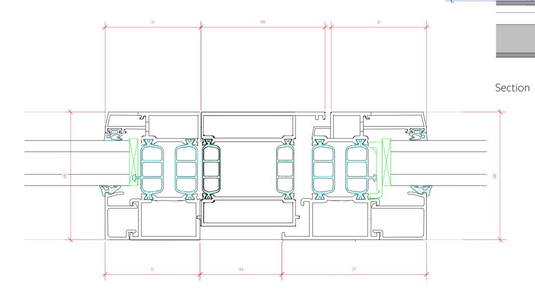
Window Detail 1:10 @ A1, 1:20 @ A3 New Crittal Style Window Aluminium profiles and plant on beads Colour RAL 7021
