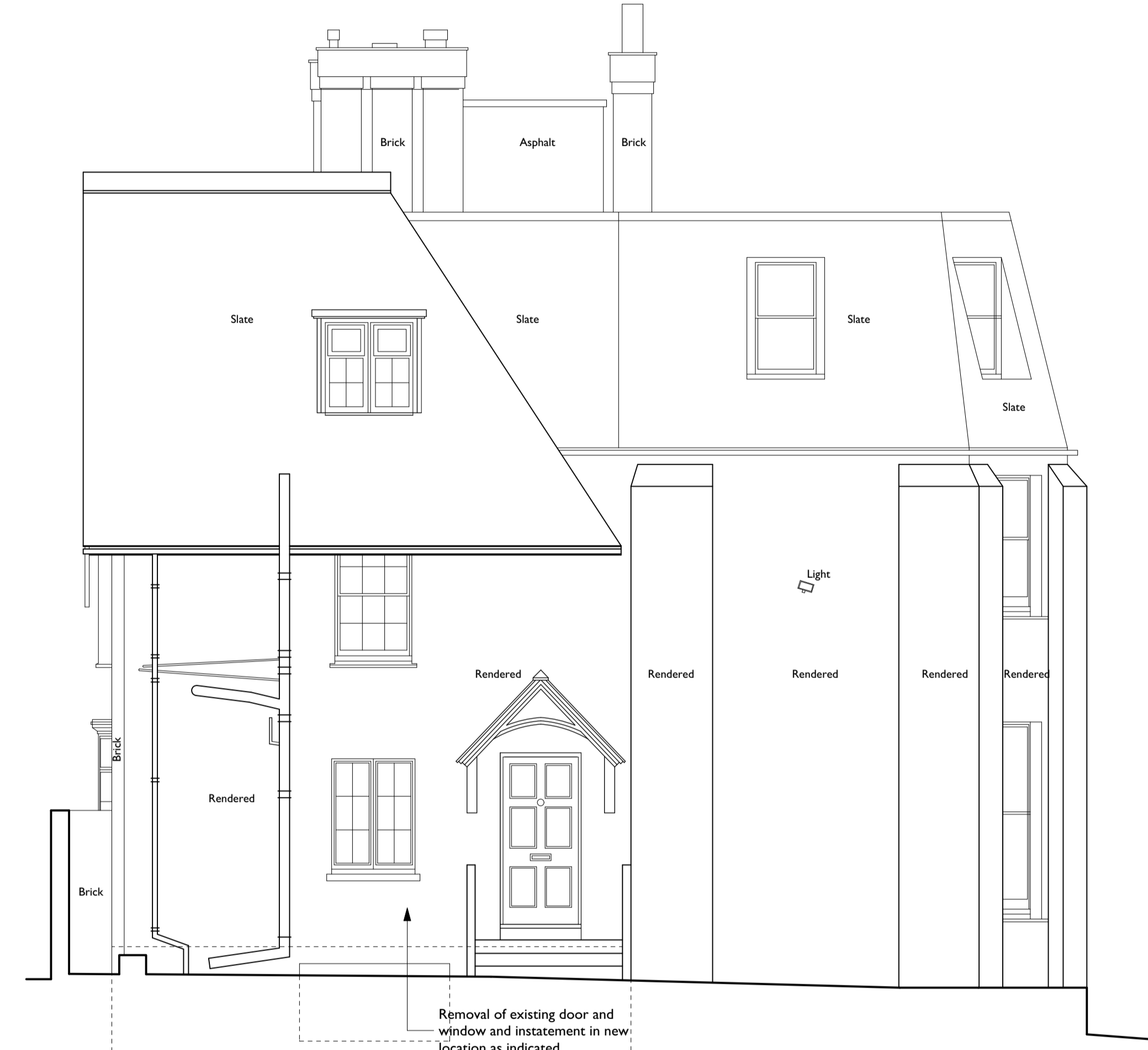
South West Elevation
