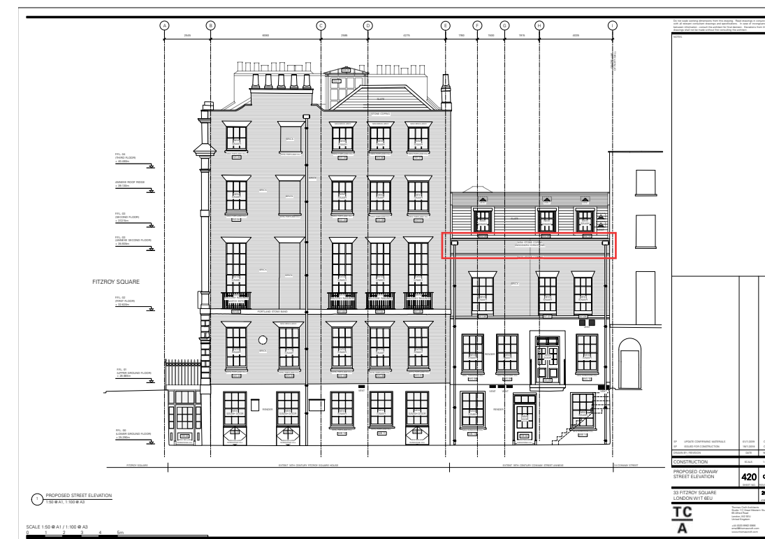
Conway St elevation - area of extended external wall using reclaimed bricks
