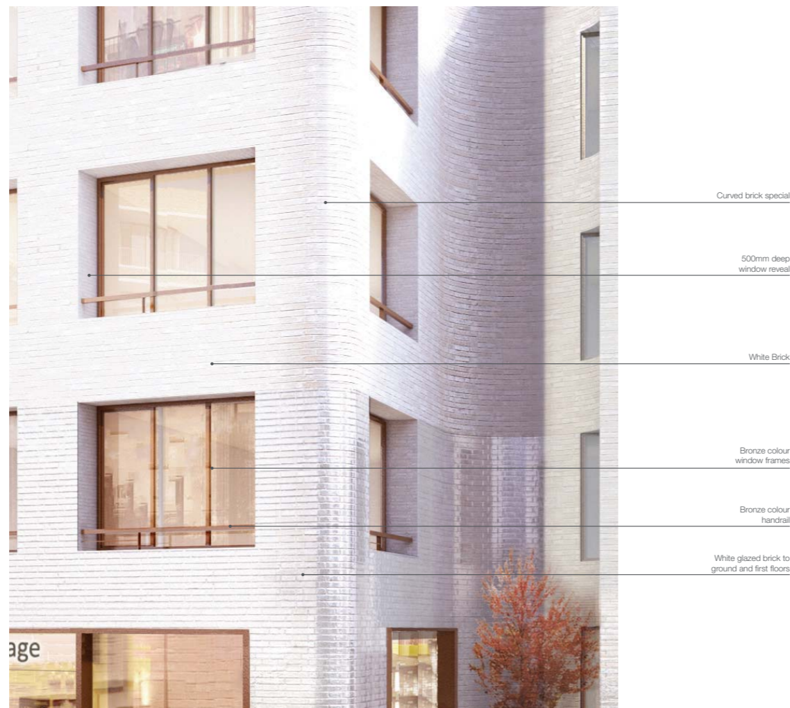
CGI image of the front elevation included in the original D&A statement shows the architectural quality of extending the brickwork corner down to ground level.
