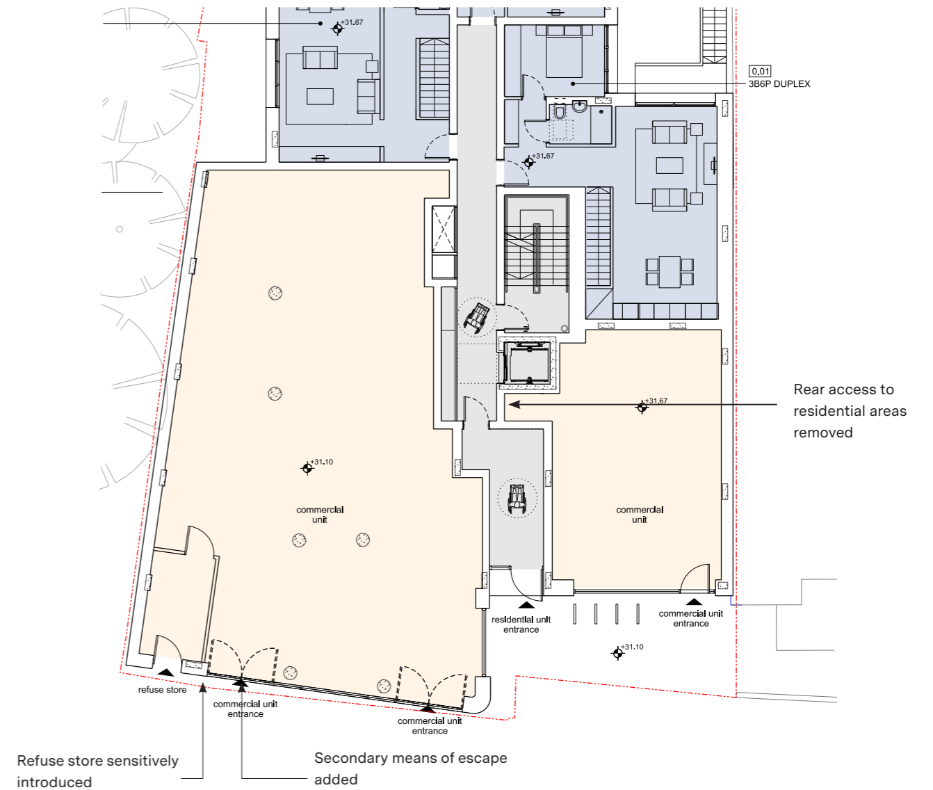
Proposed Ground Floor Plan demonstrating how the development is now compliant with fire regulations.
