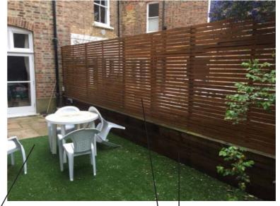
existing concrete paviors and artificial grass to be removed and replaced with ceramic tiles
