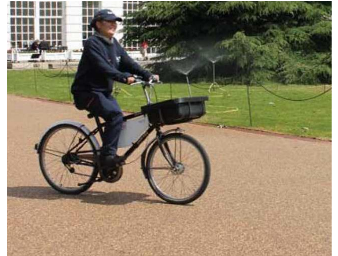
Resin-bound gravel footpath - porous surfacing to minimise impacts on tree roots
