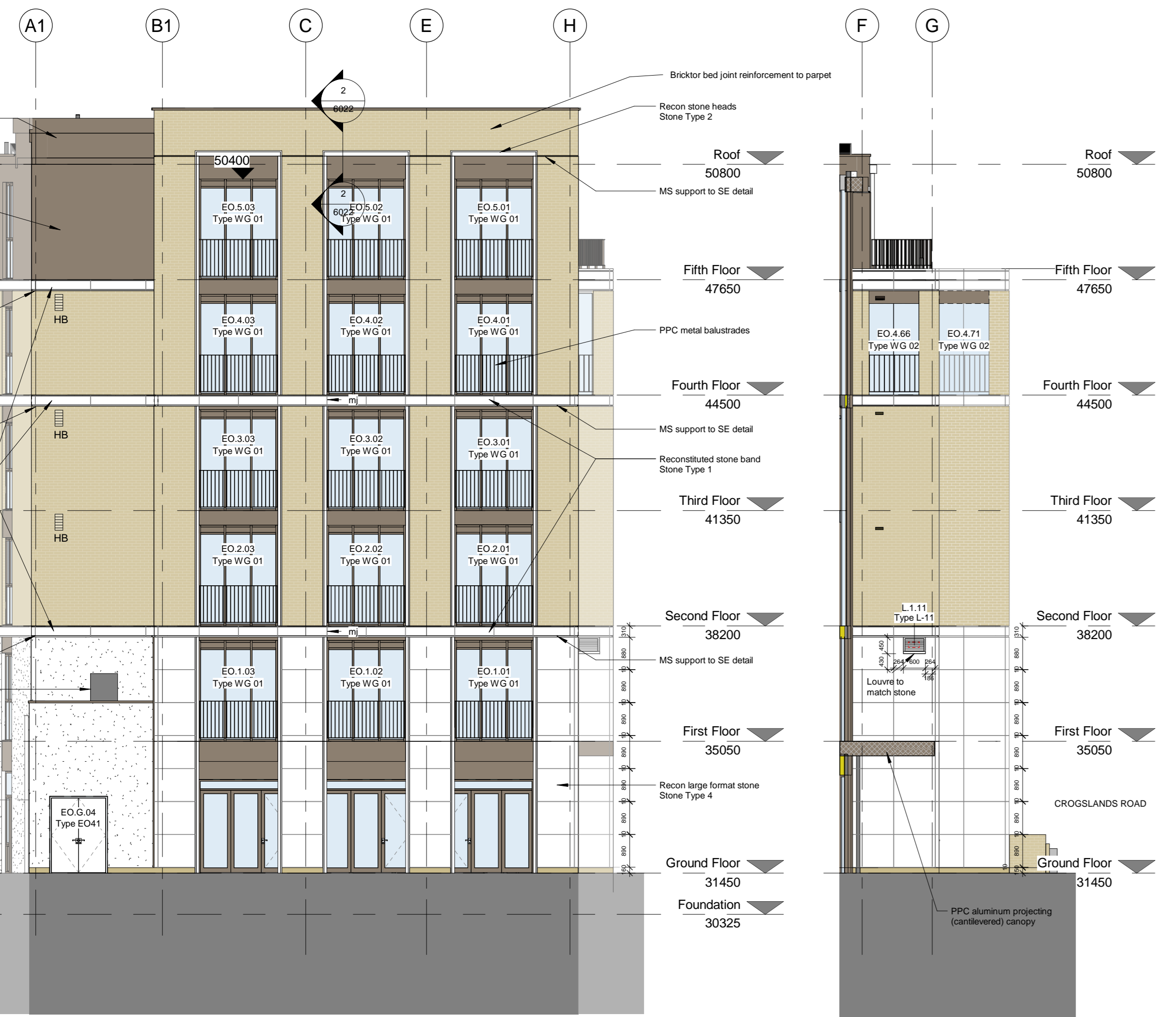
3 South Main Elevation 1:100 4 South Elevation at Stagger 1:100
