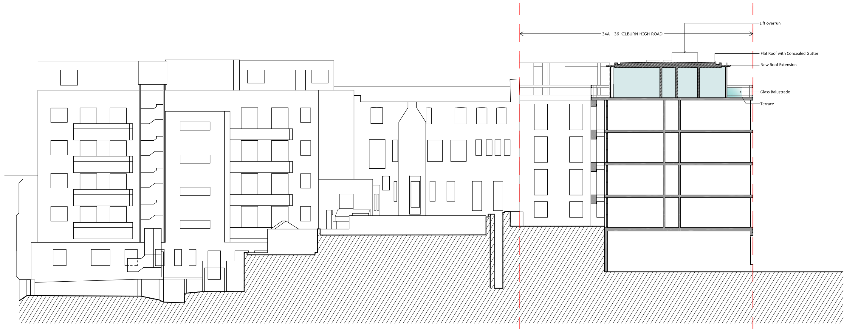
1 PROPOSED SECTION B - B 1:100 @ A1 / 1:200 @ A3
