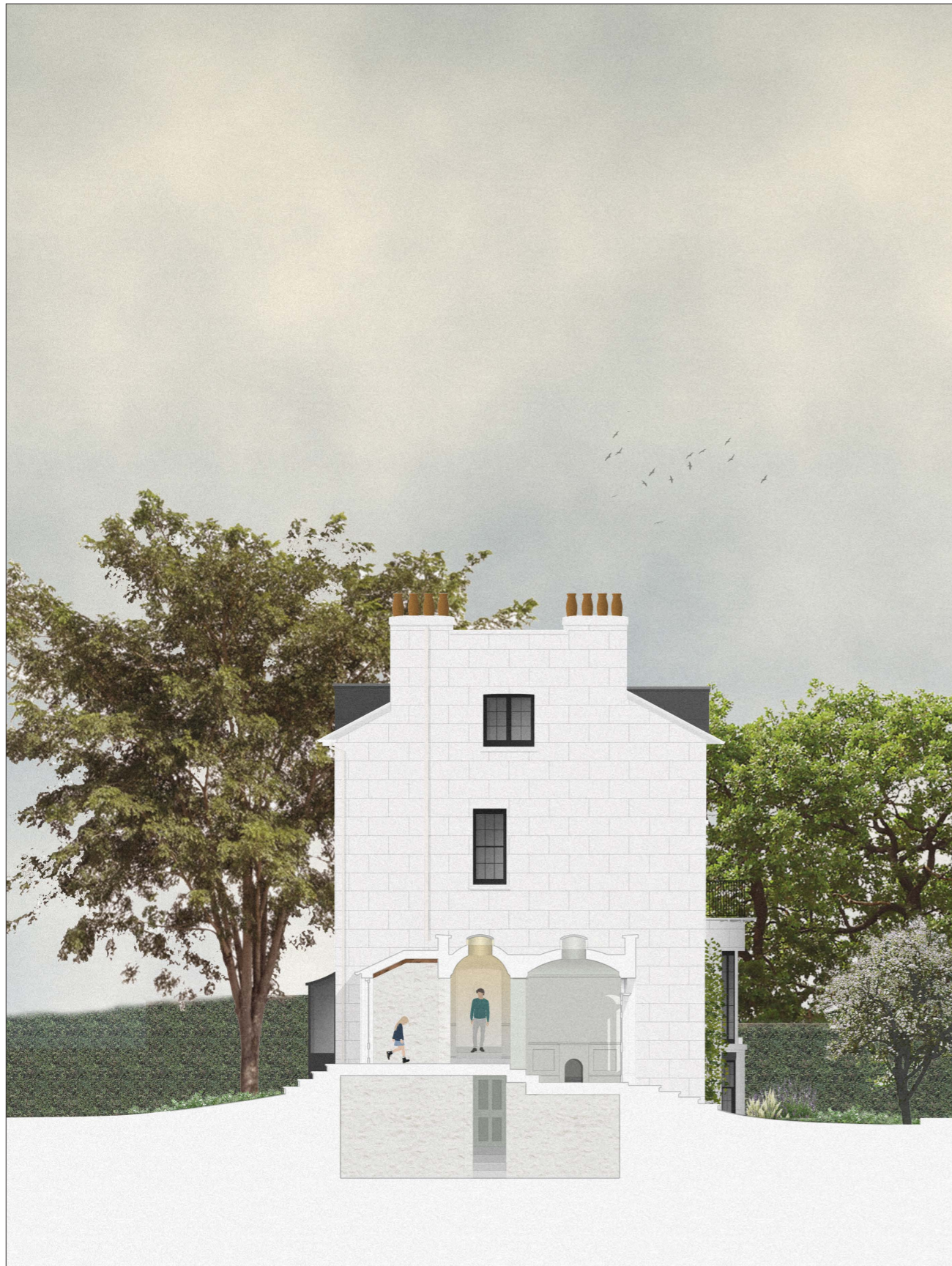
Proposed Section - through the entrance hall and new boot room extension
