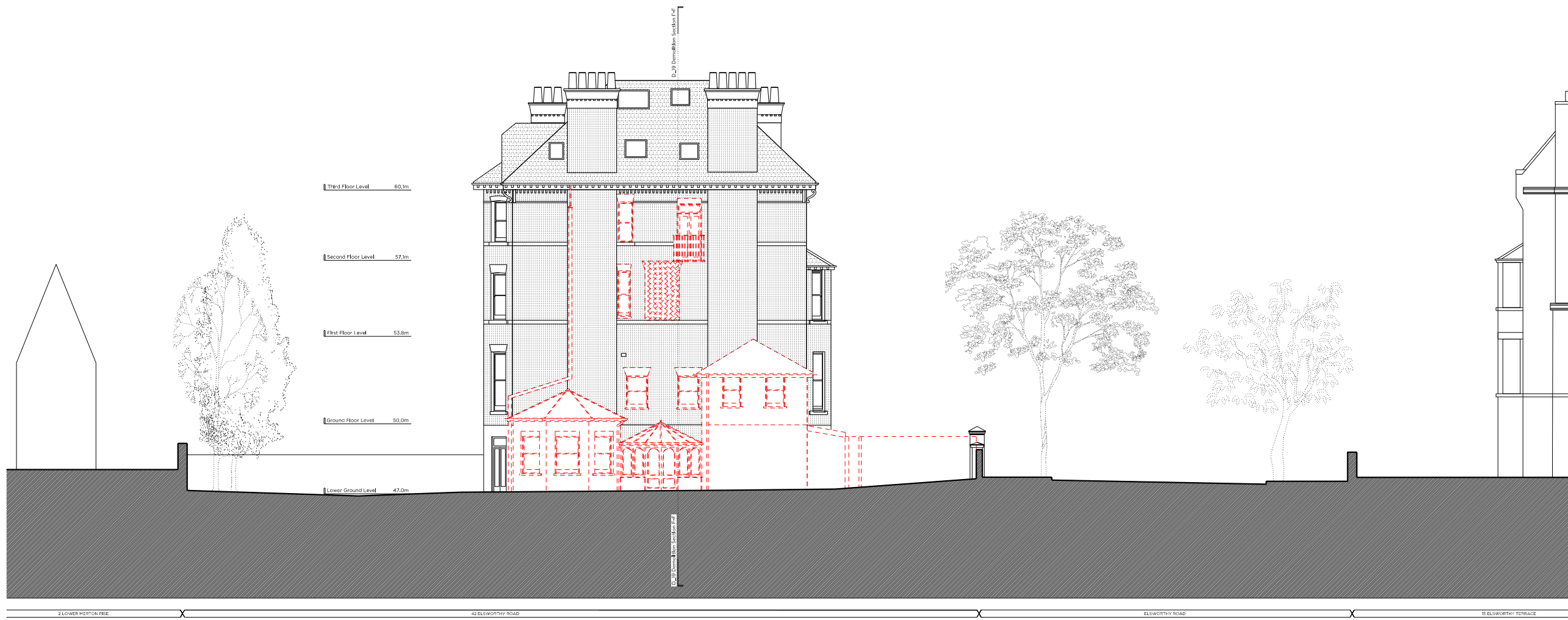
Demolition Southwest Elevation
