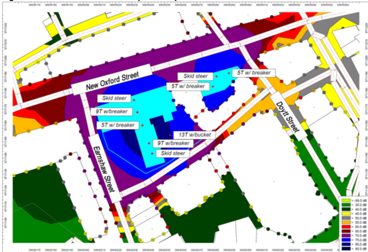
Figure 5.5.1 – Noise Contour Map for Sequence 5
