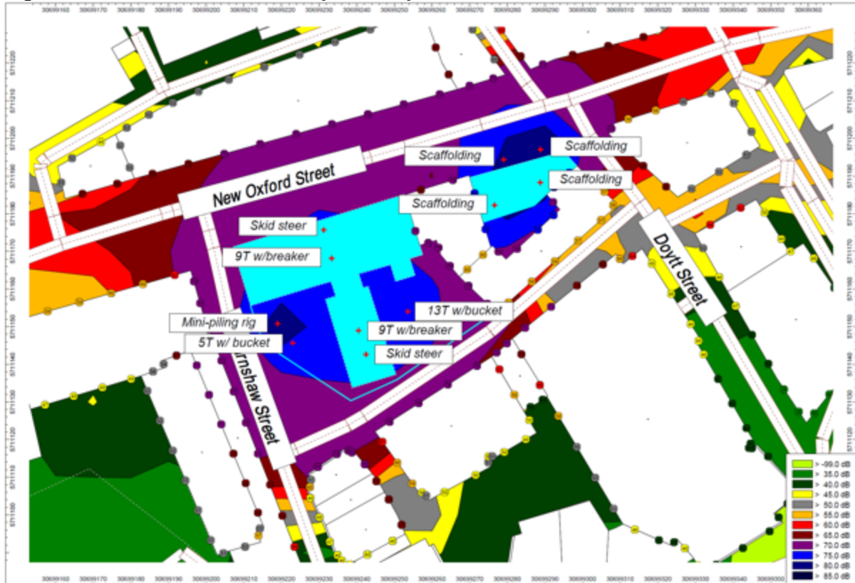
Figure 5.4.1 – Noise Contour Map for Sequence 4
