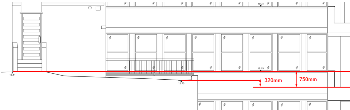
Elevation C from Matrix Surveys' measured survey (10.07.19) showing difference of between 750-320mm in external and internal floor level in Bleeding Heart Yard.
