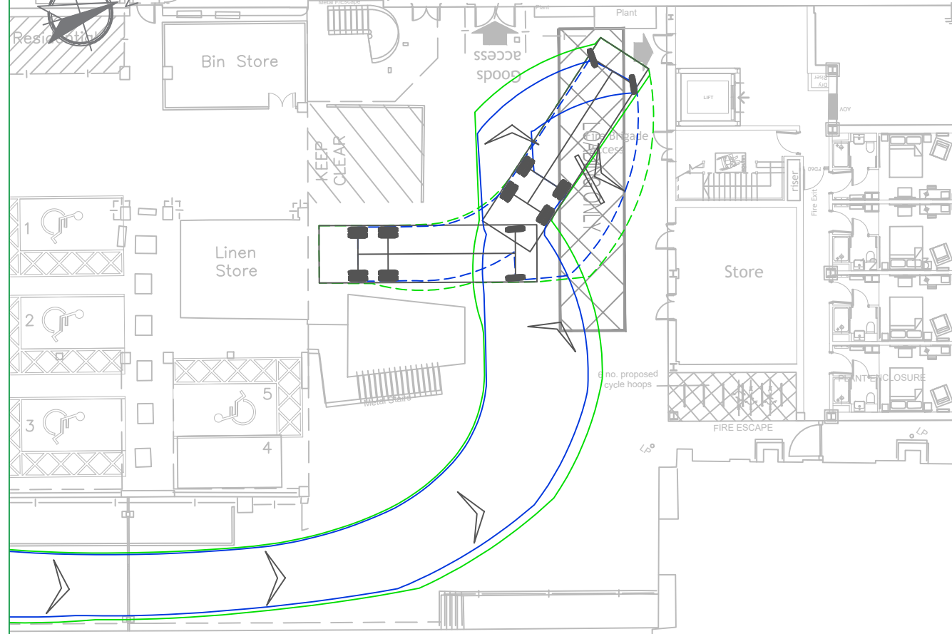
Whitbread 18t Rigid Accessing Service Yard
