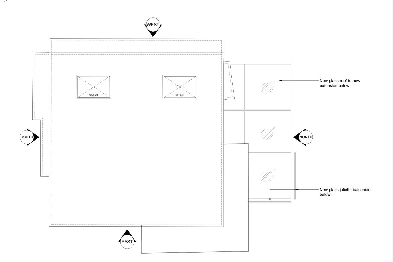
4 Roof Plan - Proposed 100 Scale 1:50@A1 / 1:100@A3
