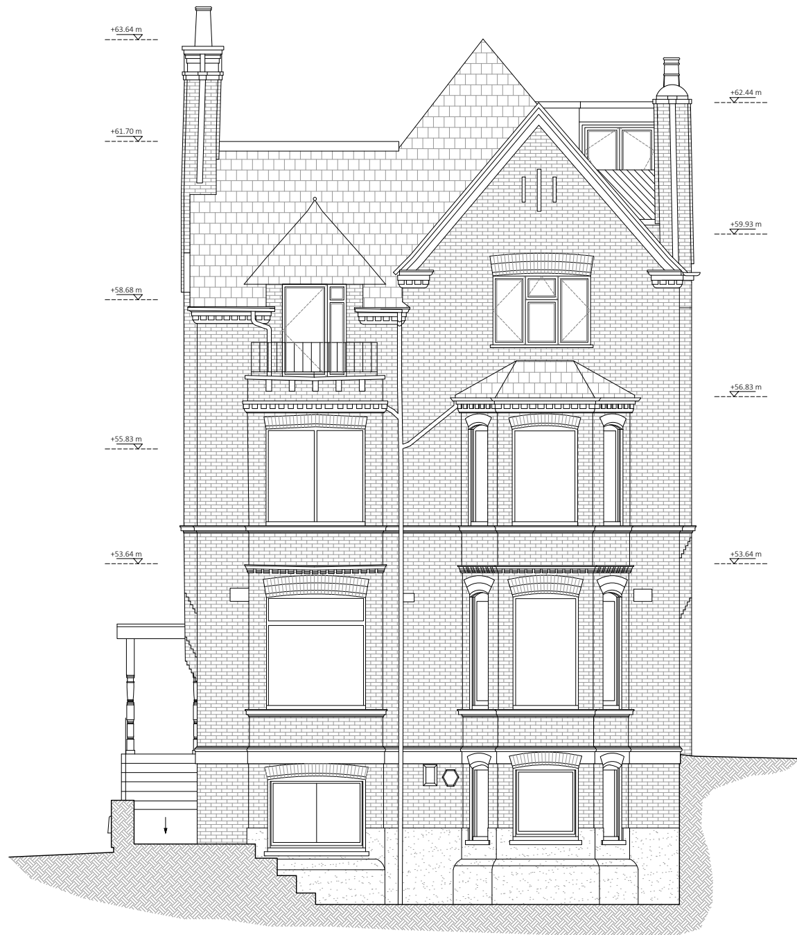
EXISTING NORTH SIDE ELEVATION
