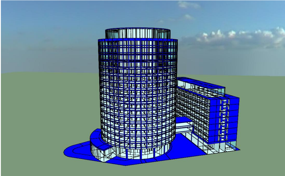
IES Thermal Model of Proposed Development: Tower Building
