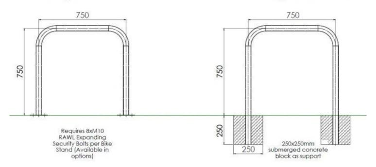
Overground fixing is ideal for very hard surfaces e.g. concrete.
